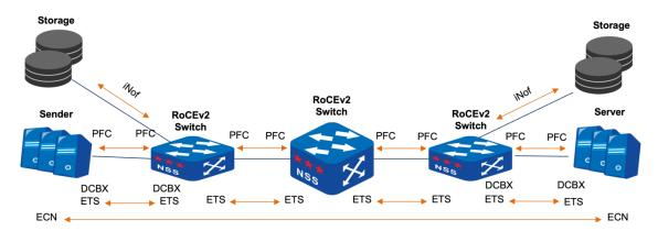
RoCEv2 is a network protocol that enables servers in data centers to perform Remote Direct Memory Access (RDMA) directly over Ethernet. RoCEv2 benefits significantly from a lossless Ethernet environment because it relies on high reliability and low latency for performance efficiency. Lossless Ethernet technology ensures that RoCEv2 can deliver its full potential benefits by avoiding the typical challenges associated with standard Ethernet communications.
