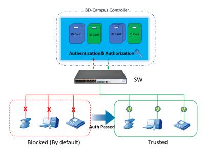
Zero Trust Access is one of the key features of Maipu BD-Campus Solution. It mainly does three things to guarantee your network is safely protected:
